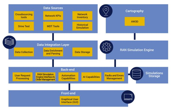
This diagram shows the range of different data sources, the ways in which these sources are integrated and enriched for presentation to the simulation engine, the cartography and RAN simulation engine, the core back-end functionality aggregating other modules and containing automation capabilities and the Graphical User Interface.
